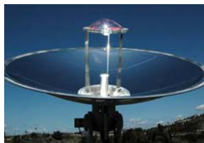
รูปที่ 1.21 : (Left) Solar concentration device, (right top) solar fiber optic system in the building, (right bottom) solar fiber optic illuminator (Proefrock,2006)
