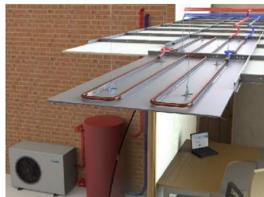
Figure C1-7-1.12 : Radiant ceiling cooling and heating system (S&P,2013)
